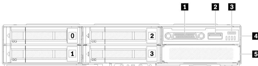
Figure 20. Four 2.5-inch drive configuration with KVM breakout module and drive bay numbering
